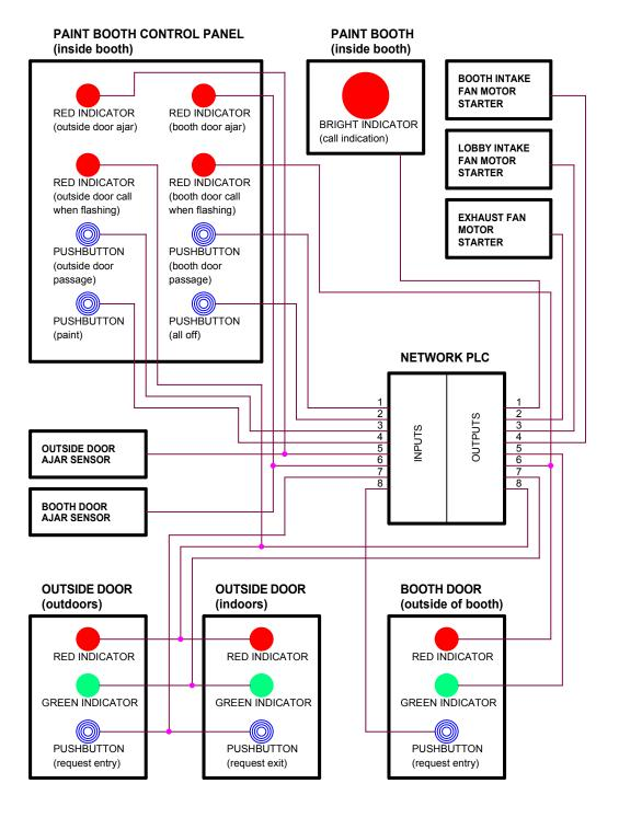
When Exhaust Fan is on, red indicators on 3 remote stations are on steady, as are the two top indicators on the Paint Booth Control Panel.
